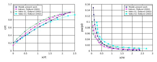
Fig. 7. Radius and wall pressure distribution.
