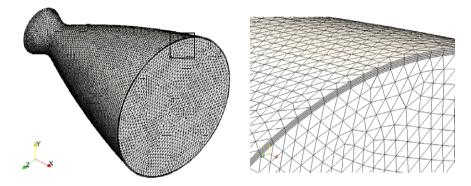
Fig. 6. Spatial discretization for the fluid and for the structure.
