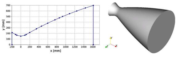
Fig. 5. Contour line and 3D model.
