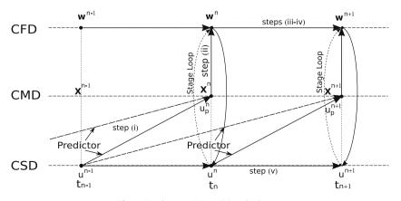
Fig. 1. Synchronous FSI partitioned scheme.
