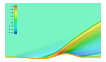
Fig. 4. Fluid and structure fields at *M* = 3.2. Colormap = fluid density, time = 1.68 s.
