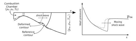
Fig. 8. Schematic deformation of the structure.
