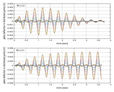
Fig. 3. Plate deflection in distributed points along plate.
