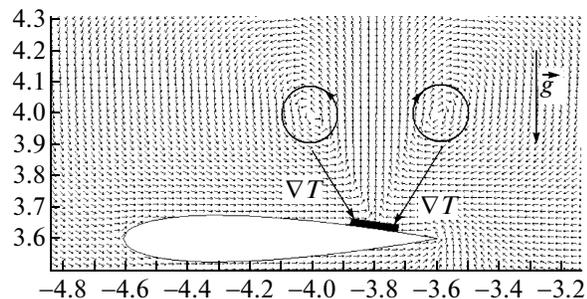
Fig. 4. (Left) Schematic diagram of simulation of convective flow, (right) vector velocity field.
