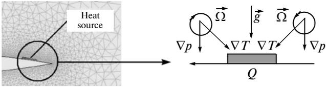
Fig. 3. (Left) Heat source position on the wing, (right) schematic diagram of formation of thermal vortices.
