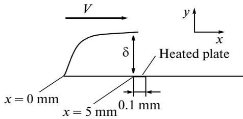
Fig. 5. Schematic diagram of calculation for supersonic flow.
