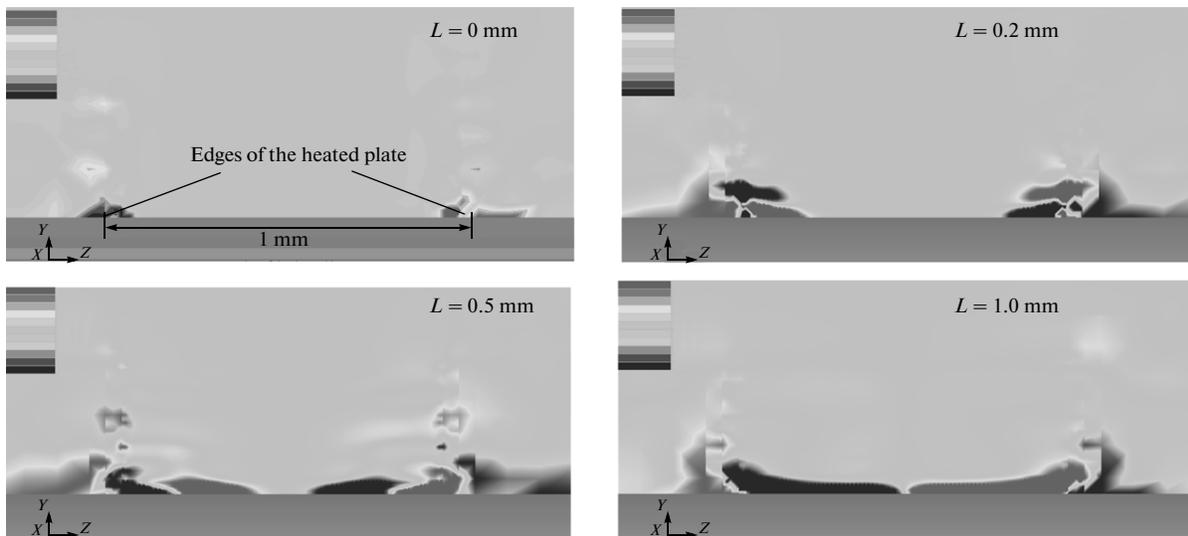
Fig. 7. Distribution of  $X$  component of vorticity along the flow at different distances  $L$  from the heated plate.
