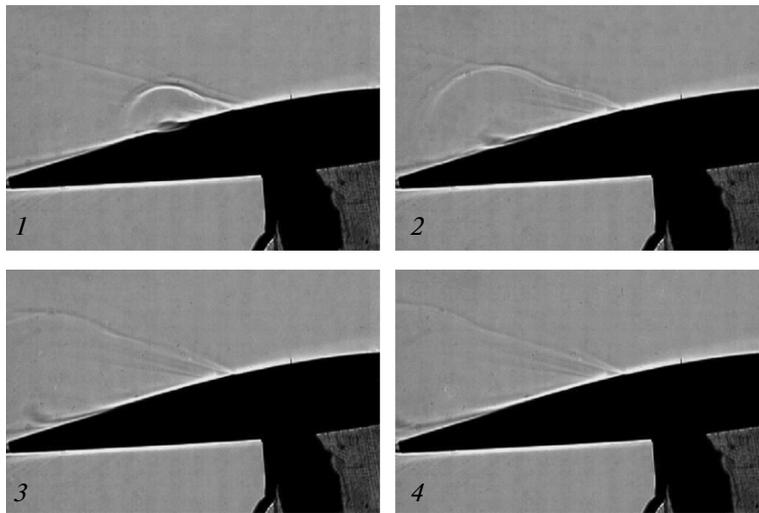
**Fig. 1.** Dynamics of extended spark discharge on the model surface. Angle of attack is 8 deg. 1—20  $\mu$ s, 2—40  $\mu$ s, 3—60  $\mu$ s, 4—70  $\mu$ s after the discharge.
