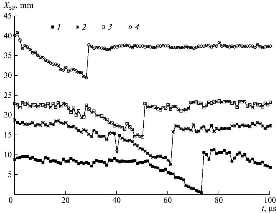
Fig. 2. Position of separation point with respect to the back end of the profile as a function of time after the discharge at different angles of attack: 1— $\alpha = 0^\circ$ , 2— $\alpha = 8^\circ$ , 3— $\alpha = 10^\circ$ , 4— $\alpha = 13^\circ$ .
