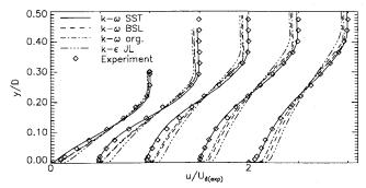
Fig. 4 Velocity profiles for Driver's adverse pressure-gradient flow at x/D = -0.091, 0.363, 1.088, 1.633, and 2.177.
