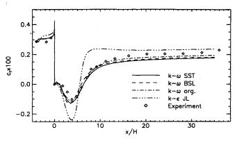
Fig. 7 Wall shear-stress distribution for backward-facing step flow.
