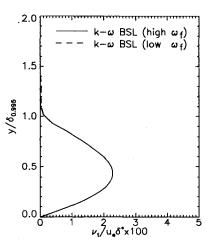
Fig. 1 Freestream dependency of the eddy viscosity for the original and the BSL  $k-\omega$  model.
