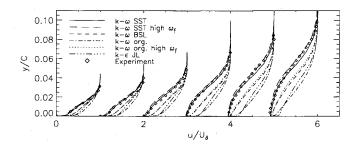
Fig. 9 Velocity profiles on the upper surface of a NACA 4412 airfoil at 13.87 deg angle of attack; streamwise stations x/c = 0.675, 0.731, 0.786, 0.842, 0.897, and 0.953.
