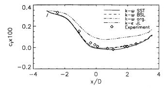
Fig. 3 Wall shear-stress distribution for Driver's adverse pressuregradient flow.
