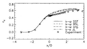
Fig. 2 Wall pressure distribution for Driver's adverse pressure-gradient flow.
