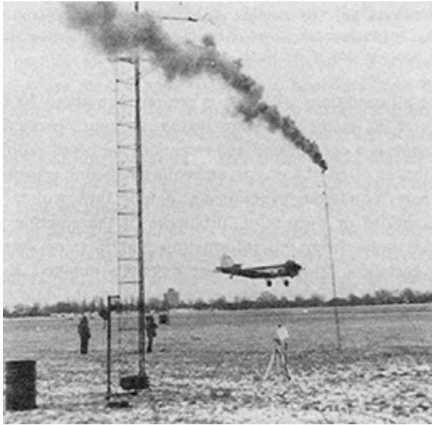
Fig. 1.5 Turbulent motion in a smoke trail generated to indicate wind direction for landing tests.
