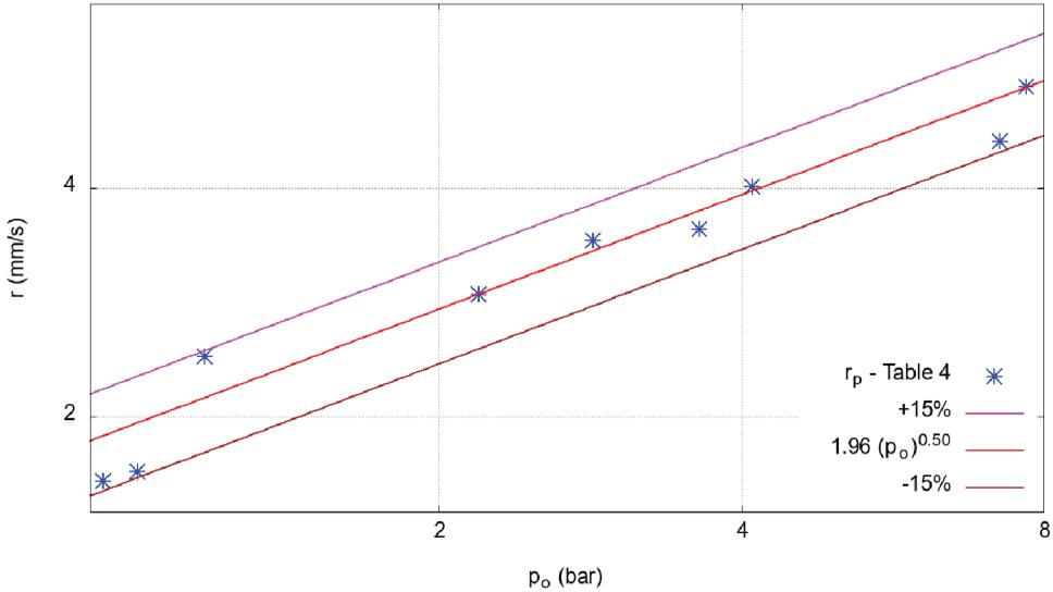
**Figure 5.** KNSu burning rate versus combustion pressure.
