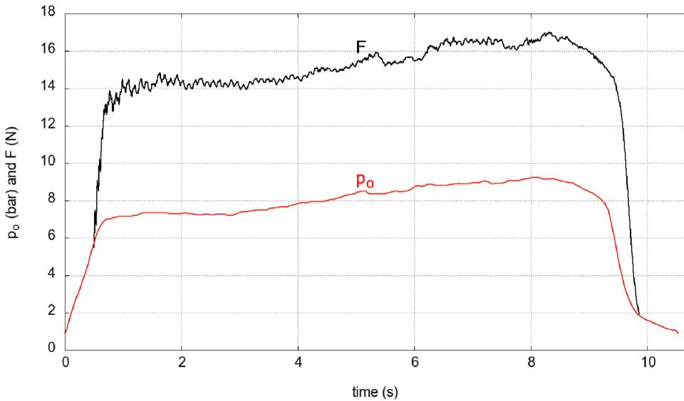
**Figure 4.** Thrust and pressure curves for test 44.
