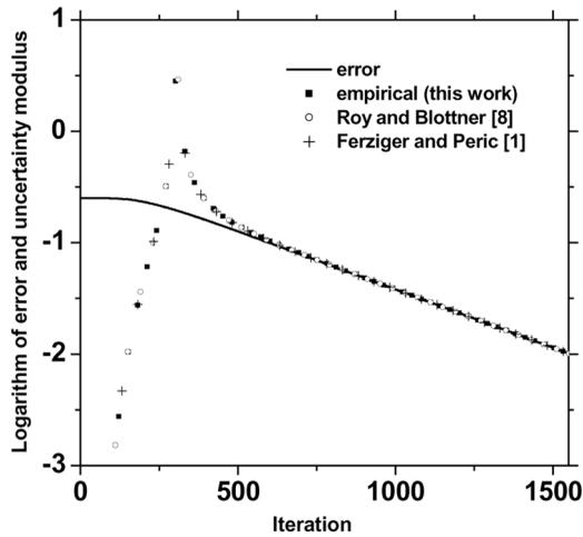
**Figure 3.** Error ( $E$ ) and uncertainty ( $U$ ) for  $\Lambda(L/2, L/2)$ , Problem 2, grid of  $65 \times 65$  nodes, without multigrid.
