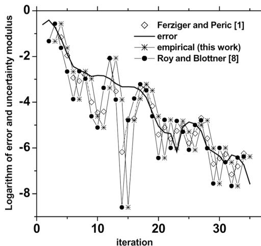
**Figure 4.** Error ( $E$ ) and uncertainty ( $U$ ) for  $\Lambda(L/2, L/2)$ , Problem 2, grid of  $65 \times 65$  nodes, with multigrid.
